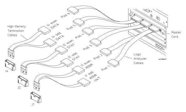
Chapter 4: Connecting the Logic Analyzer to the HTI board Connecting the Logic Analyzer to the Motorola HTI board 5
